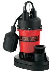
**Tethered Float Switch** – The tethered float switch is a buoy device attached with a cord that raises and lowers with the water level, activating a switch inside the pump telling it to turn on, drain the water, and then turn off once water level has subsided. Debris can't hinder operation therefore this switch is used for sump, effluent or sewage applications. Replacement switches are available.
