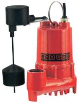
**Vertical Float Switch** – The vertical float switch is a buoy device attached with a rod that raises and lowers with the water level, activating a switch attached outside the pump telling it to turn on, drain the water and then turn off once the water level has subsided. This style allows for installation in confined areas. This switch is designed for sump applications only. Replacement switches are available.
