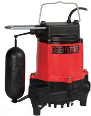
**Snap-Action Float Switch** – The snap-action float switch is a contractor-preferred switch built into the pump. It's designed for confined areas, but unlike a traditional vertical float switch, debris can't hinder operation so it is suitable for sump and effluent applications. The switch features a solid float that will never become waterlogged.
